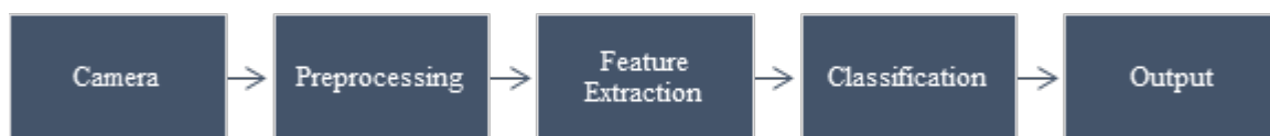
Fig. 1: Embedded vision processing pipeline showing camera input, preprocessing, feature extraction, classification, and output stages.
